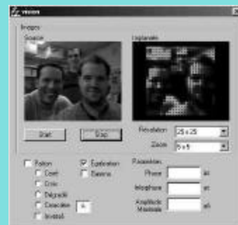
Figure 3: The user interface of the external controller prototype presenting the real image and its corresponding 25x25 pixelized one that a blind patient could see using the implantable device.
