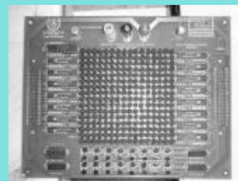
Figure 2: The display part of the non-implantable prototype of the EVCS emulating a 16x16 matrix of microelectrodes model.
