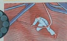
A worker loads the TAT-1 cable in the hold of the Monarch, as the ship prepares for the journey across the North Atlantic. The Monarch was the largest cable ship afloat at that time with four cable holds each 270 ft in diameter.
