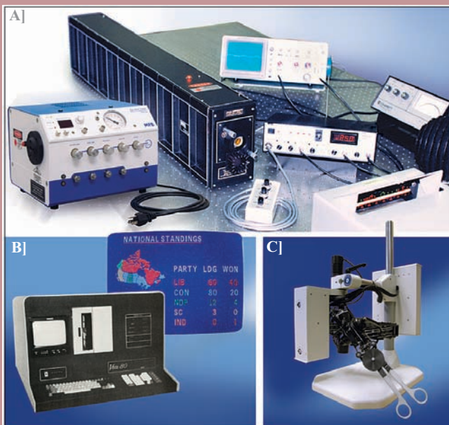
Figure 2: MPB products primarily from the earlier years: A) Early MPB lasers: mini-excimer and CO 2 ; B) VISTA 80 graphics generator for television broadcasting; C) Freedom 7 force feedback hand controller (present).
