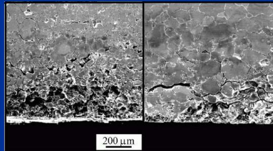
Grain de-cohesion due to inter-granular corrosion
