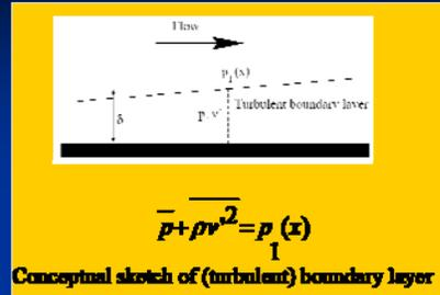
Correlating temporal pressure field to cavitation inception (fully developed boundary layer flow).
