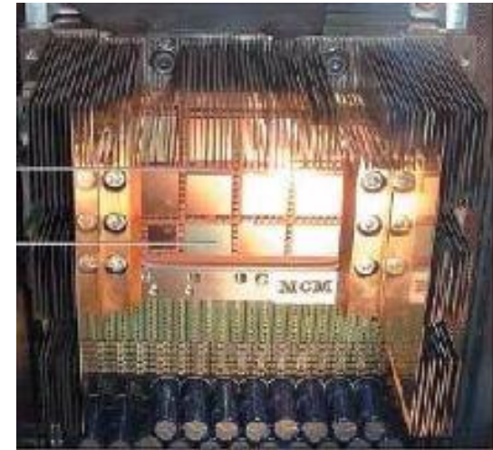
z9 MRU cooling with aircooled backup mode
