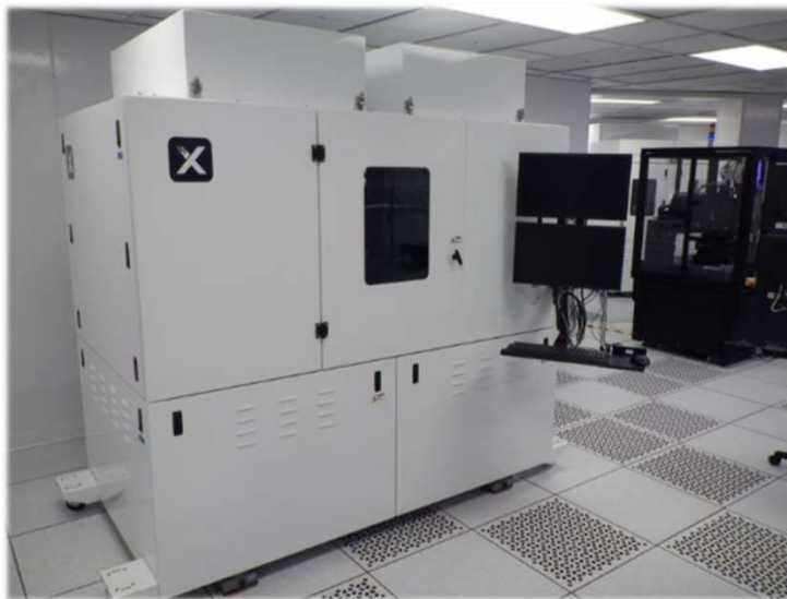
Transfer-printer designed to populate 300mm diameter wafers
