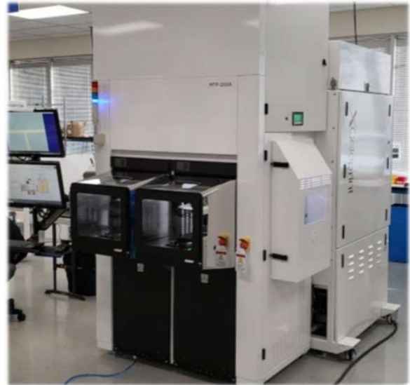
Transfer-printer with automated substrate handling
