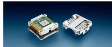
Figure 4. Mid-board optics modules shown here provide the key to a high-density interface.
