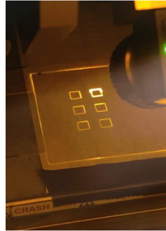
Cavity drilling process
