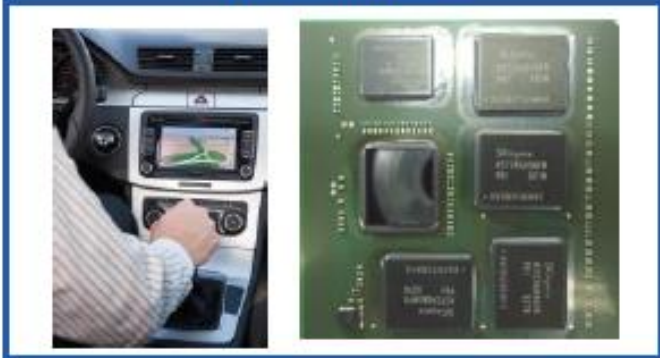
42.5 x 42.5 mm, Infotainment, Processor + DDR
