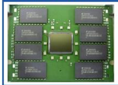
55 x 72 mm, Network Switch, ASIC + Memory
