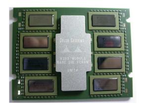
bare die ASIC + CSP1 memories to alleviate the burden placed on the Plated Thru Hole (PTH) based PCBs
