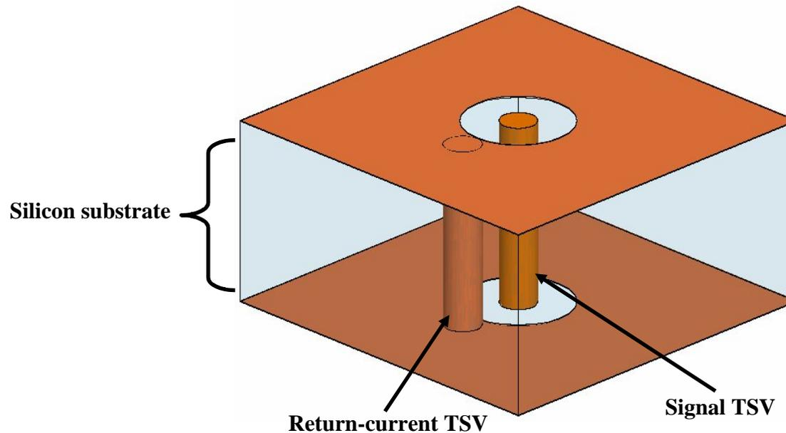
3D model of signal and return-current TSVs
