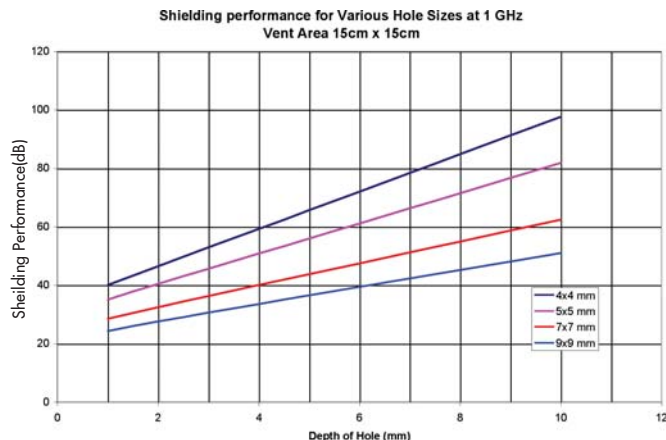
Figure 2 Shielding performance at 1 GHz for various hole sizes and thicknesses.
