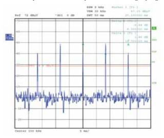
Fig. 3. Result of PRF measurement for EUT7.
