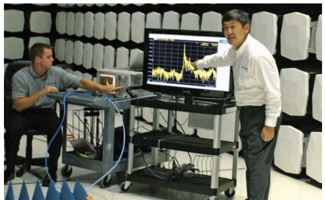
Zhong Chen points out the VNA display that shows how to pick out site irregularities.
