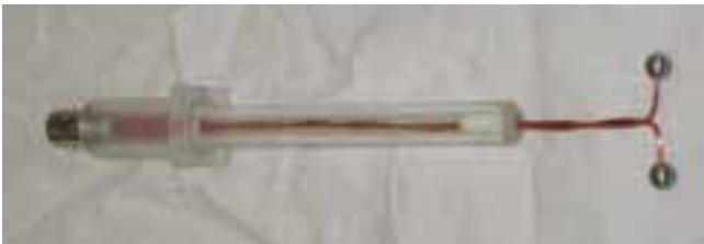
Fig. 2. The sensor holder. The copper wires are insulated and twisted from the spheres up to the twin-lead connector at the top.
