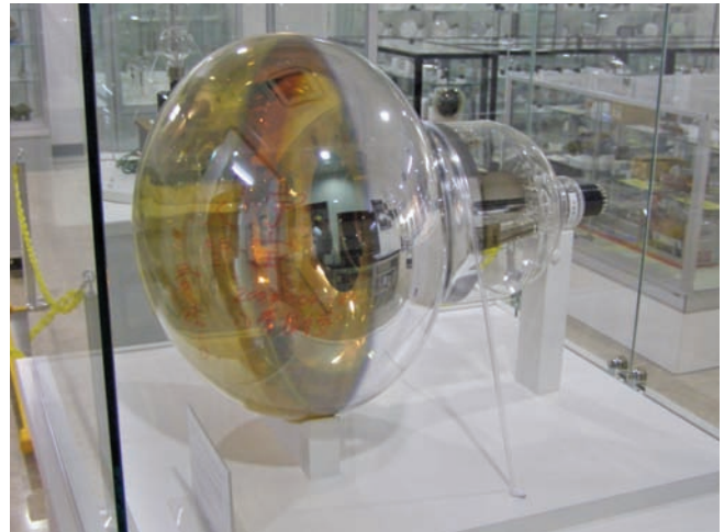
A photomultiplier tube for neutrino detection used at the world famous Kamiokande Observatory in Nagano, Japan.
