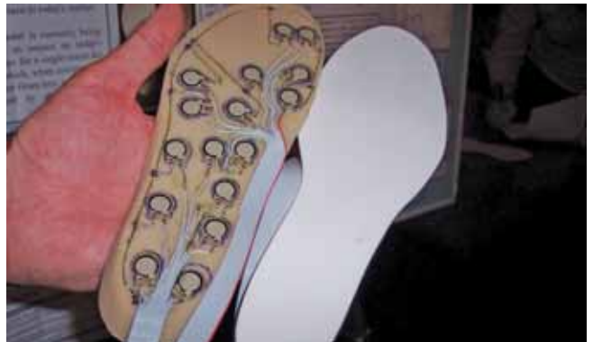
A close up of the biosensor insole at the Milwaukee IEEE Section event.
