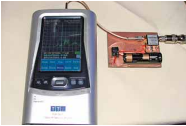
Ken Wyatt's inexpensive spectrum analyzer that utilizes a Palm Pilot for a display shown during his presentation to the Los Angeles Chapter in June.
