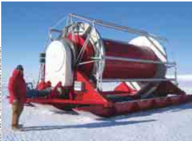
Hose Reel for the Enhanced Hot Water Drill at the South Pole.
