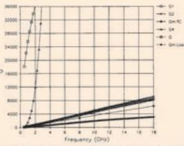
Fig. 5. Calculated and measured Q for the FAA cavity with a circular aperture of radius 1.4 cm and three salt-water spheres of radius 6.6 cm. Q1, Q2, and Q4 are calculated from wall loss, absorption, and antenna reception. Q3 from aperture leakage is off scale.
