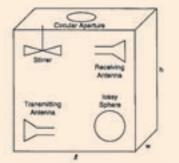
Fig. 4. Rectangular cavity with a circular aperture, a mode stirrer, receiving and transmitting antennas, and lossy sphere(s).
