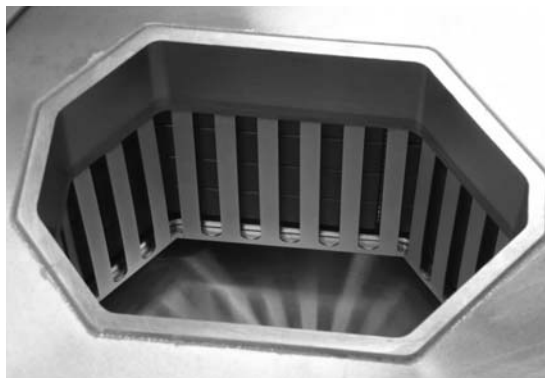
Figure 5. Picture of the RF shield for the upgraded bellows section at one end of the BaBar detector. Note the large gaps between the fingers. The HOM absorbing tiles can be seen behind the shield fingers.
