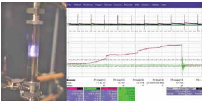
Figure 5: Voltage and current waveforms obtained from a 200 W cold plasma Hydrogen chamber using ethanol as fuel
