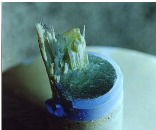
fig 18 Brittle Fracture - Mechanical Failure of the fibreglass core; photos [8].
