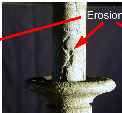
fig 9 Examples of damage on the sheath/shank: Erosion (Left hand photo [9]).
