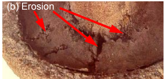
fig 4 Examples of damage at the polymer/fitting interface (seal): (a) Core Exposure due to Splitting/Cutting [14], and (b) Erosion [8].
