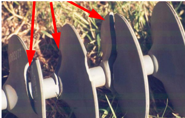
fig 15 Examples of damage to sheds: (a) Splitting/Cutting which reduces the creepage distance by >10%[14], and (b) Tracking/Carbonising on insulator sheds.
