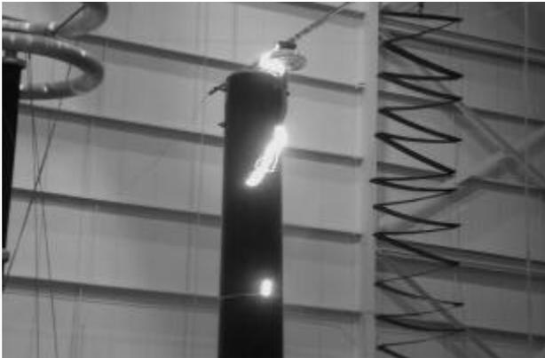
Fig. 6. The 35 kV porcelain pin insulator plus fiberglass pole, the tested pole length is 3 feet. The discharge developed on the surface of insulator and both sides of the pole's surfaces.
