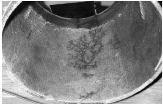
Fig. 15. The tracking appeared on the inside surface after 6.5 hours aging in salt fog with 25 kV/ft electrical stress, recorded leakage current is about 75~85 mA.
