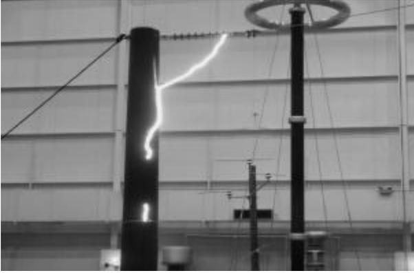
Fig. 5. The 35 kV polymer suspension insulator plus fiberglass pole, the tested pole length is 6 feet. The discharge didn't develop on the surface of insulator, but appeared in the air and on both sides of the pole's surfaces.
