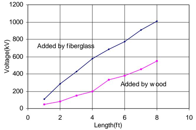
Fig. 11. The Added CFO voltages by fiberglass and wood poles to 15 kV polymer suspension insulators, wet condition and positive impulse.
