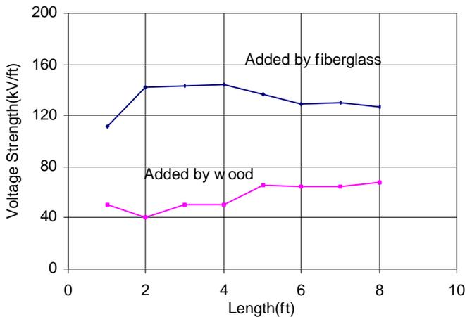
Fig. 14. The Added CFO voltage strengths by fiberglass and wood poles to 15 kV polymer suspension insulators at wet condition and positive polarity.
