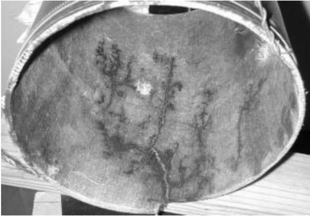
Fig. 16. The tracking appeared on the inside surface after 4 hours aging in salt fog with 25 kV/ft electrical stress, recorded leakage current is about 50~75 mA.
