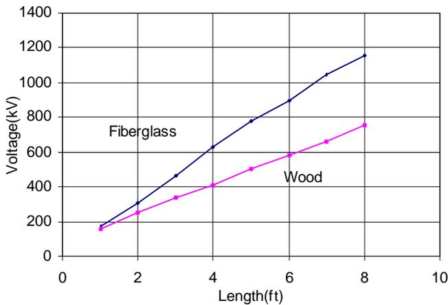
Fig. 2. The CFO voltages of the fiberglass and wood poles under wet conditions and positive polarity.
