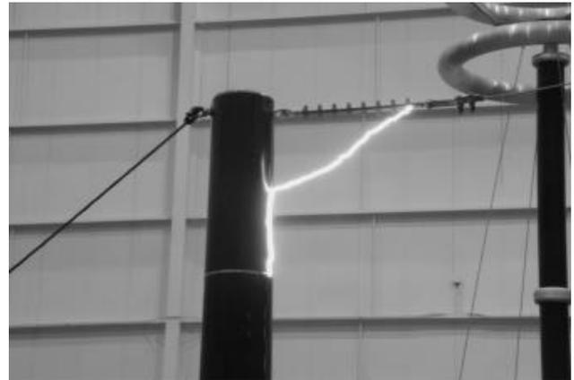
Fig. 4. The 35 kV polymer suspension insulator plus fiberglass pole, the tested pole length is 2 feet. The discharge took place in the air and on the surface of the pole.
