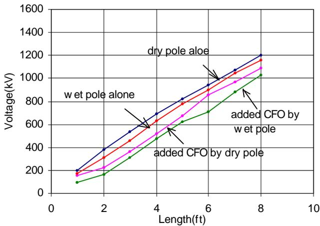
Fig. 10. The CFO voltages of fiberglass pole and the Added CFO voltages to 35 kV polymer suspension insulator, wet condition and positive impulse.
