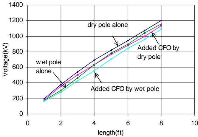
Fig. 9. The CFO voltages of fiberglass pole and the Added CFO voltages to 35 kV porcelain pin insulator, wet condition and positive impulse.
