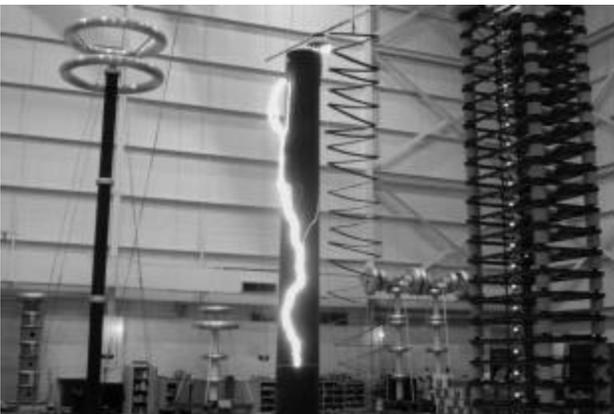
Fig. 7. The 35 kV porcelain pin insulator plus fiberglass pole, the tested pole length is 8 feet. The discharge developed on the surface of insulator and the pole.
