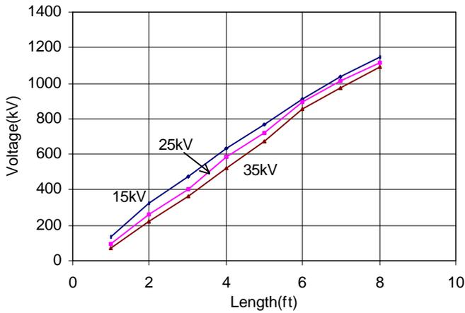
Fig. 8. The Added CFO voltages to 15 kV, 25 kV, and 35 kV polymer suspension insulators, dry condition and positive impulse.
