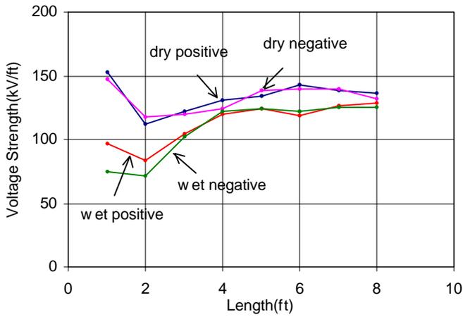
Fig. 12. The Added CFO voltage strengths by fiberglass pole to 35 kV polymer suspension insulators.
