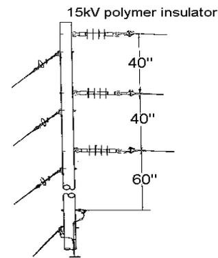
Fig. 1. Typical configuration of distribution line pole structure, the pole serves as a second insulation component.
