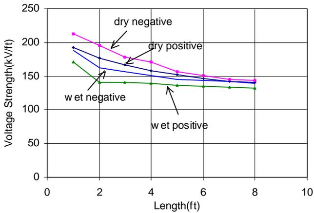
Fig. 13. The Added CFO voltage strengths by fiberglass pole to 35kV porcelain pin insulators.
