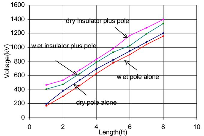
Fig. 3. The CFO voltages of 35 kV polymer suspension insulators plus the fiberglass pole and the CFO voltage of fiberglass pole, under dry and wet conditions, positive lightning impulse.
