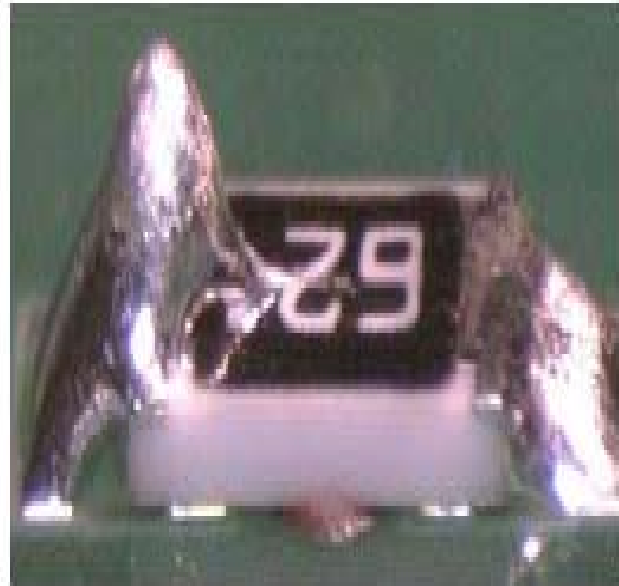
Iciding of SMD using No-clean ROLO Flux
