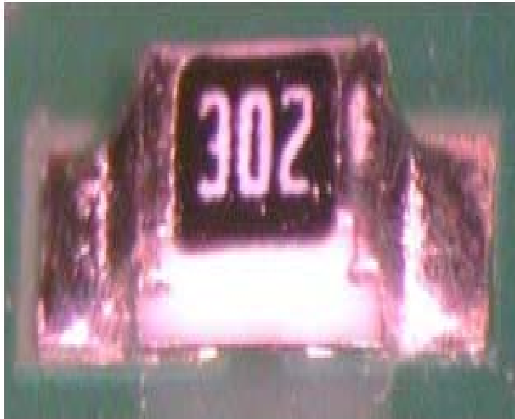
Well soldered SMD bottom-side
