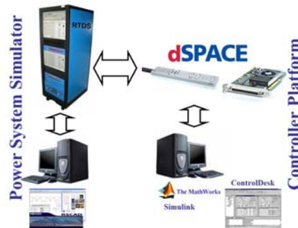
Figure 2. Hardware Configuration in Real-Time Implementation
