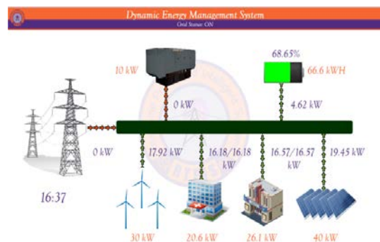
Fig. 1: Microgrid system with Dynamic Energy Management System
