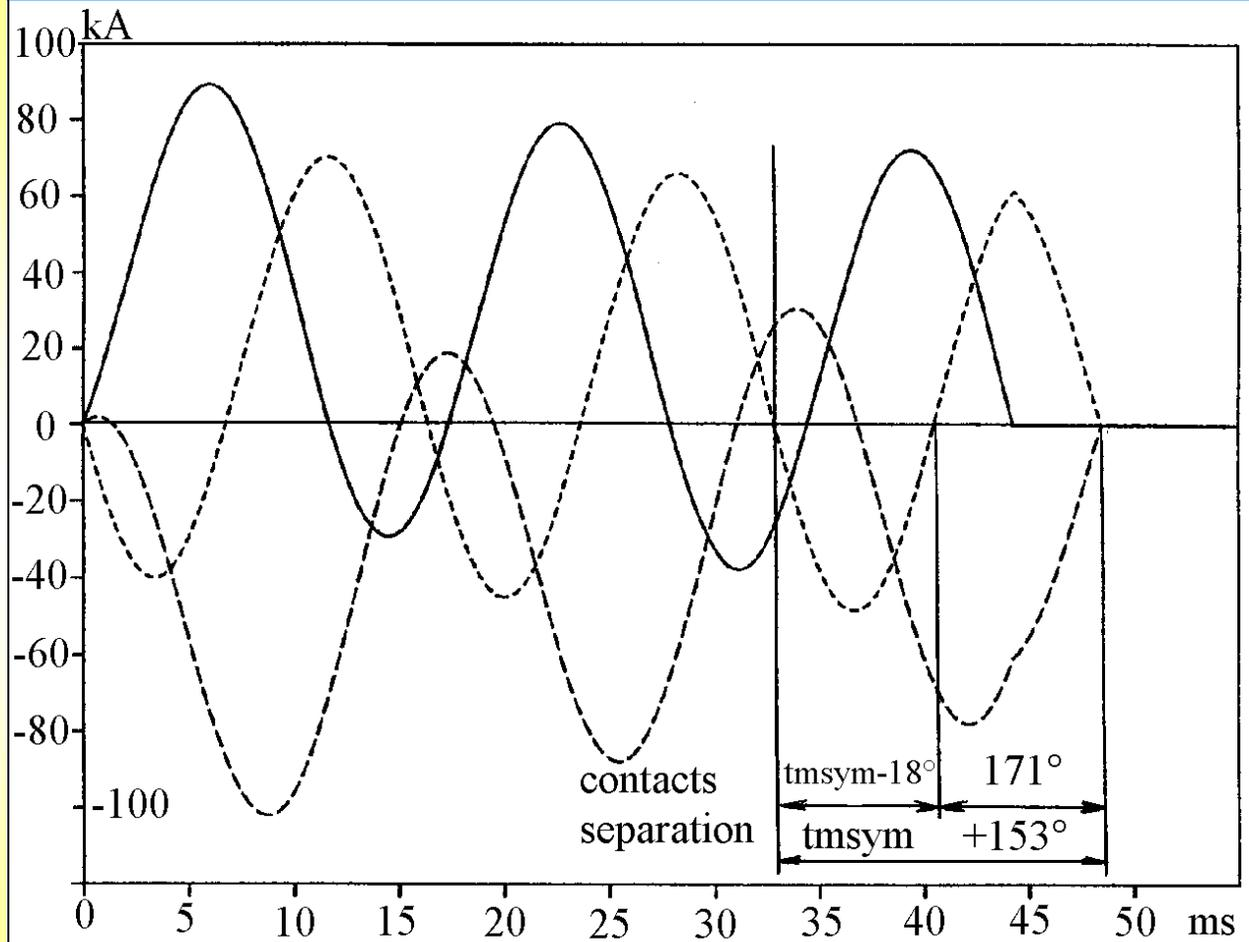
**THREE-PHASE SHORT-CIRCUIT TESTING OF HIGH-VOLTAGE
