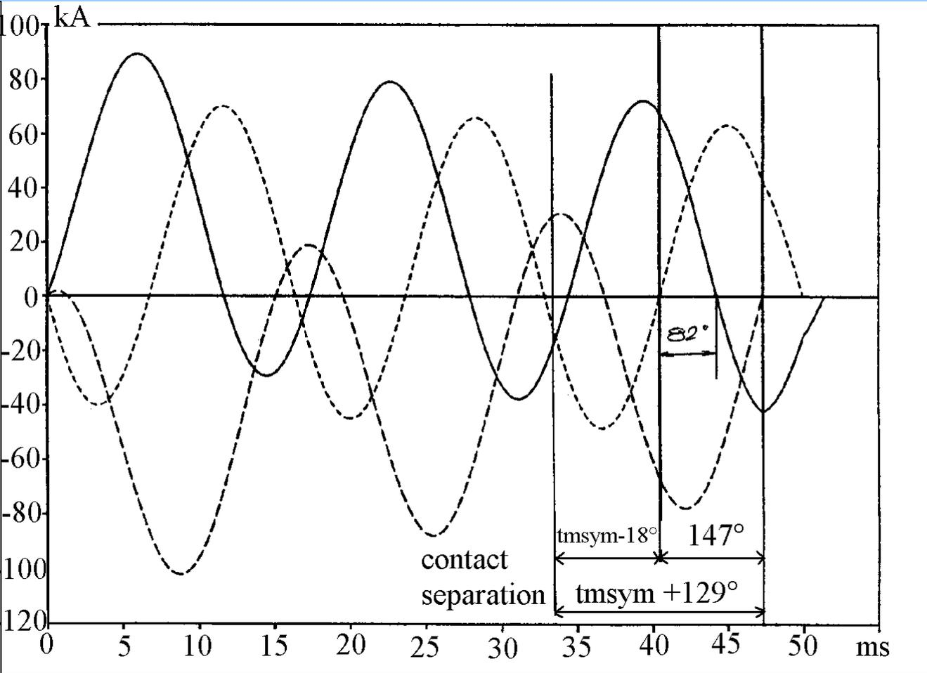
**THREE-PHASE SHORT-CIRCUIT TESTING OF HIGH-VOLTAGE
