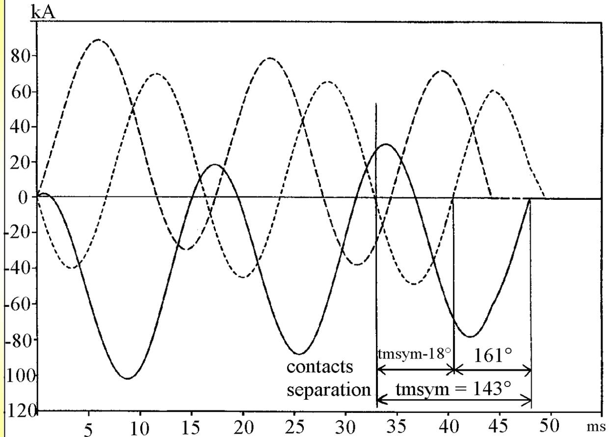
**THREE-PHASE SHORT-CIRCUIT TESTING OF HIGH-VOLTAGE
