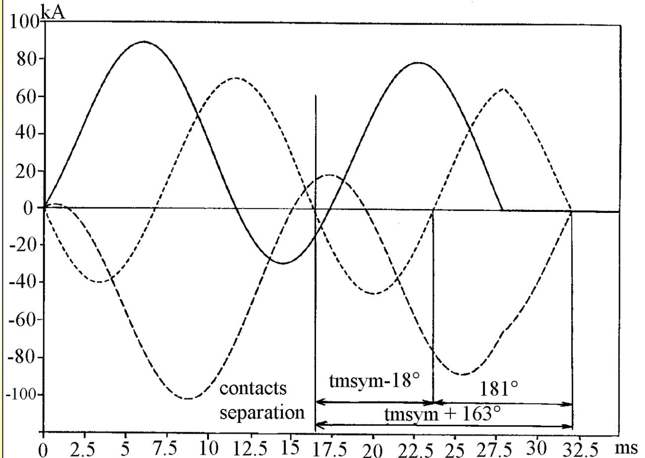
**Asymmetrical currents during 3-phase short-circuit interruption of 40 kA-60Hz by 3-cycle circuit breaker with  $k_{pp}=1.5$ . Interruption after a major extended loop by the second pole to clear.**
