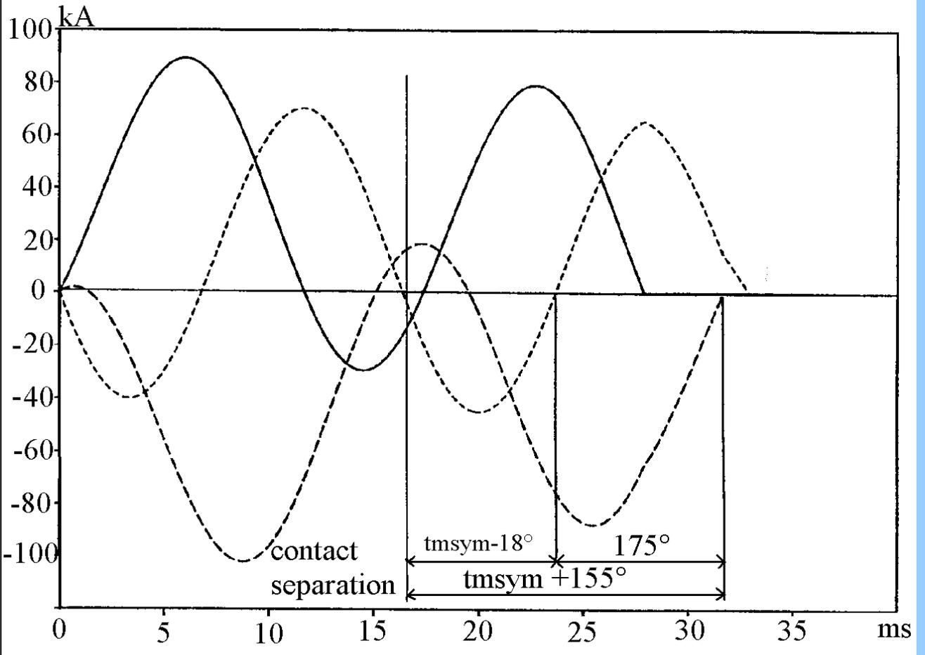
**Asymmetrical currents during 3-phase short-circuit interruption of 40 kA-60Hz by 3-cycle circuit breaker with  $k_{pp}=1.3$ . Interruption after a major extended loop by the second pole to clear.**
