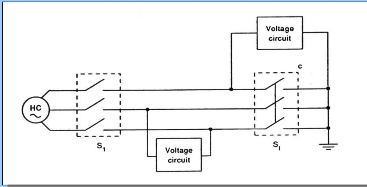
**THREE-PHASE SHORT-CIRCUIT TESTING OF HIGH-VOLTAGE
