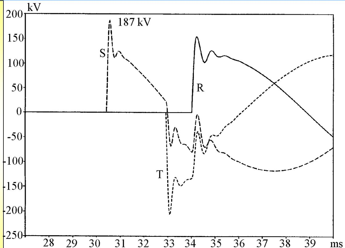
**Asymmetrical currents during 3-phase short-circuit interruption of 40 kA-60 Hz by 3-cycle circuit breaker with  $k_{pp}=1.3$ . Interruption of the first pole to clear factor after a major loop.**
