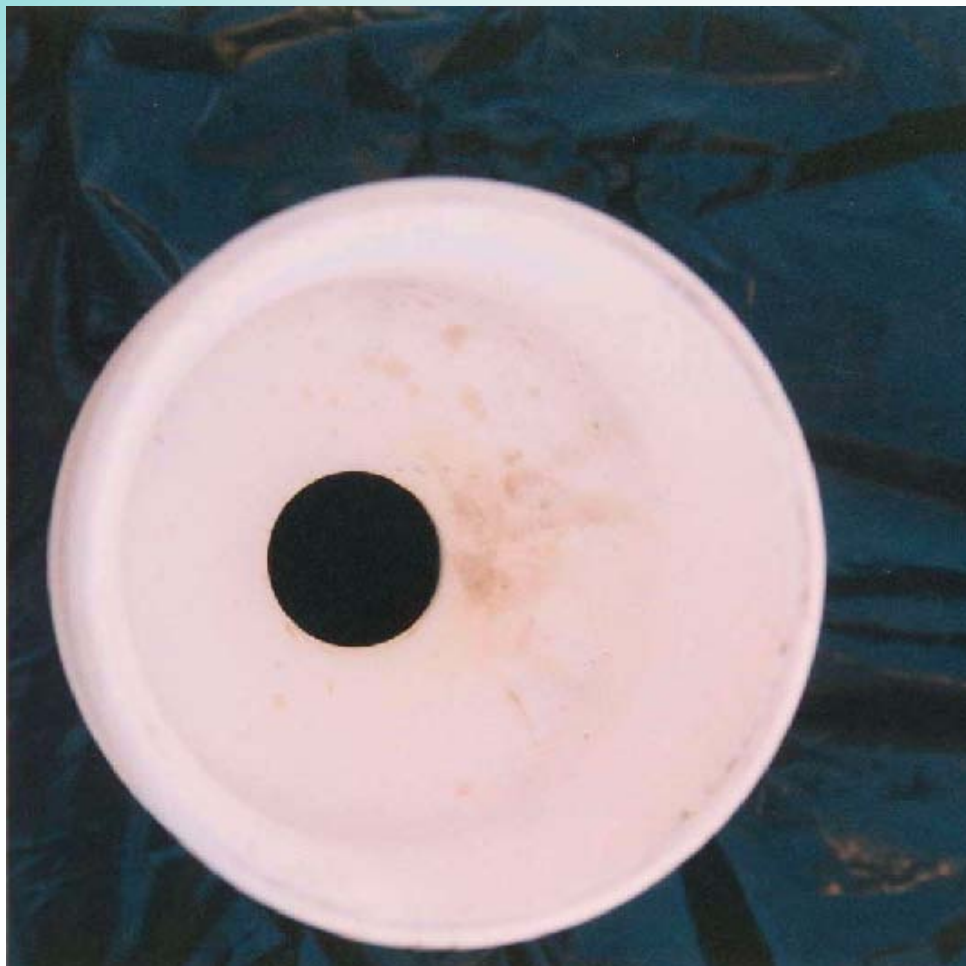
Fig 4. New nozzles were installed in circuit breaker of Fig.3 and after 650 operations were de-assembled. These were the effects.
