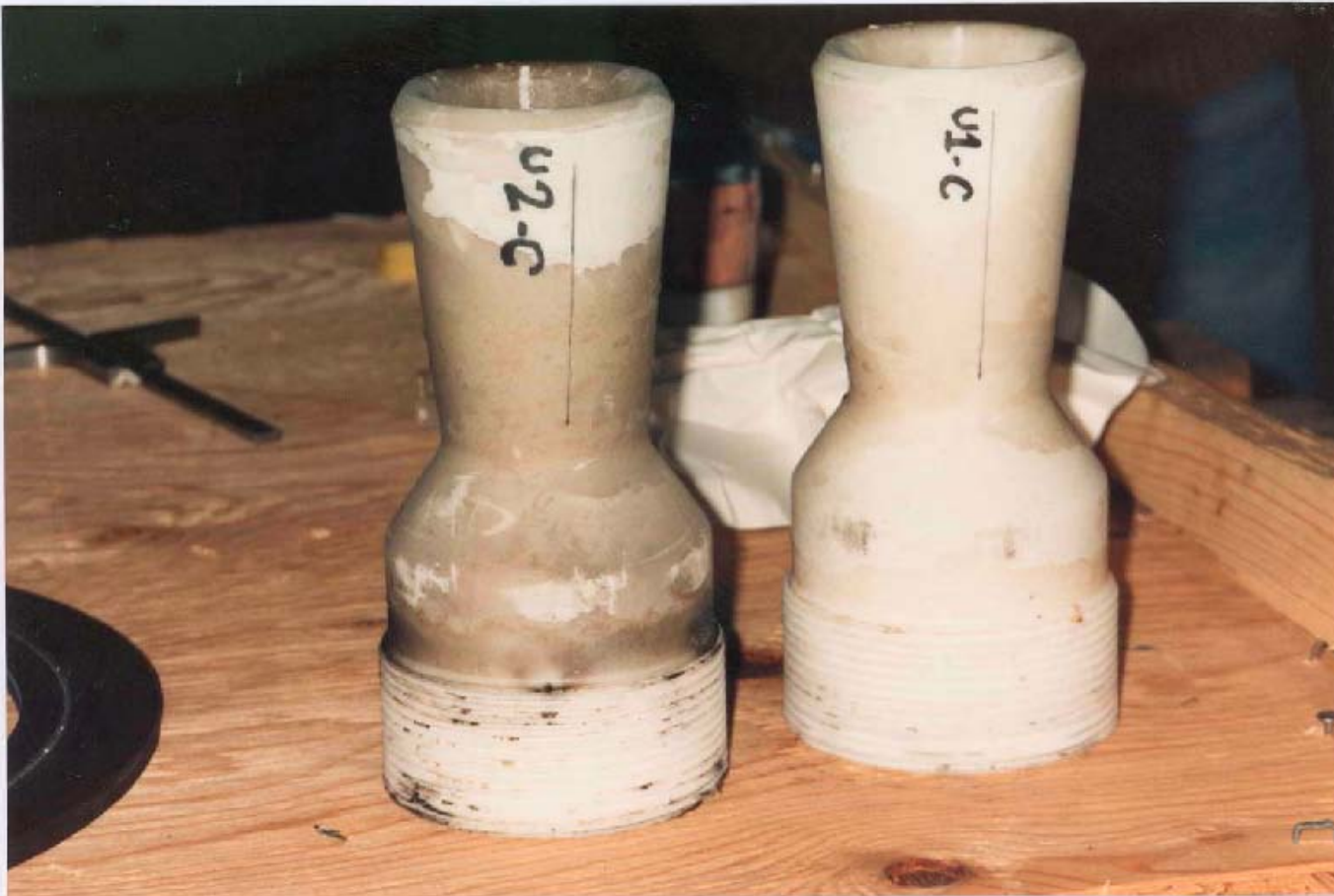
Fig 1. Nozzles of a SF6 circuit breaker after 1500 operations with uncontrolled opening switching
