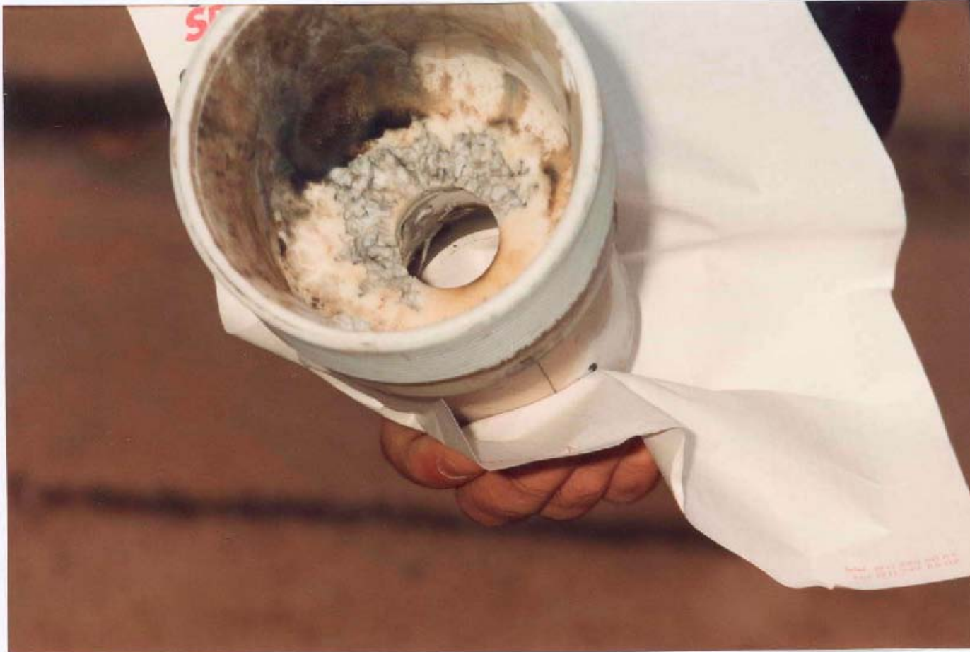
Fig. 3. Nozzles with puncturing effect after 1500 operations with uncontrolled opening switching
