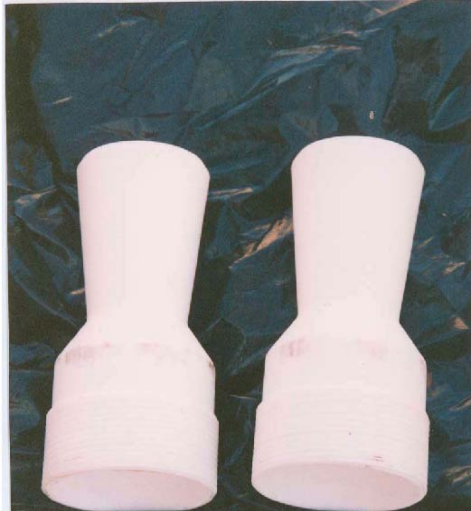
Fig 2. Same nozzles than Fig.1 after 650 operations with controlled opening switching
