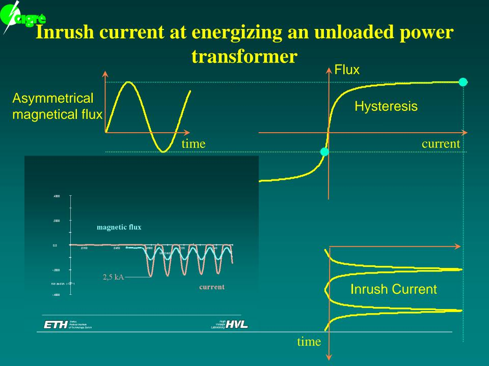
Energization current of a power transformer with controlled switching considering the remanence flux
