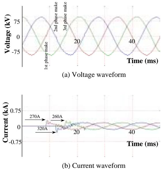
Fig.12 (b) Waveforms of the 10<sup>th</sup> capacitor energization
