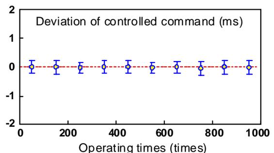
Fig.9 Deviation of the controlled switching commands issued by the controller during the consecutive operations
