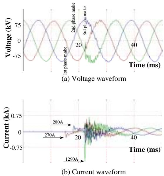
Fig.12 (a) Waveforms of the 1st capacitor energization
