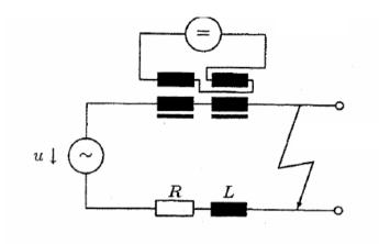
Transducer Principle (e.g. Inductive Type SCFCL ("Saturated Iron Core"))
