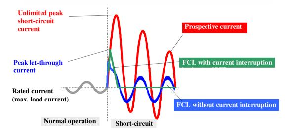
Typical Current Waveforms Due to a Fault
