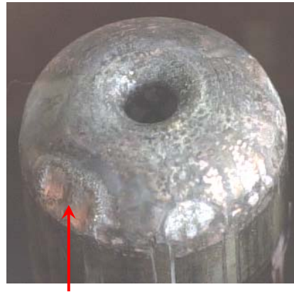
Damaged fixed arcing contact
