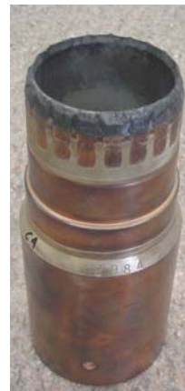
Seriously damaged moving contact (M4)
