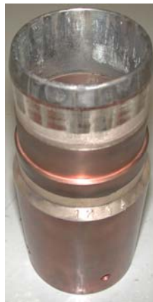
Worn moving contact (M3)
