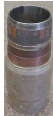
Slightly worn moving contact (M2)
