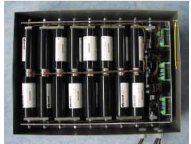
Switch box including 2600F ultracapacitors
