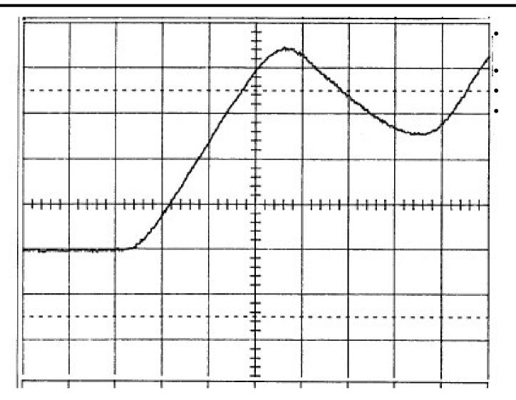
Used in the same way as the polaroid pictures Only few channels Not so much points Time resolution ok for short line fault TRV's
