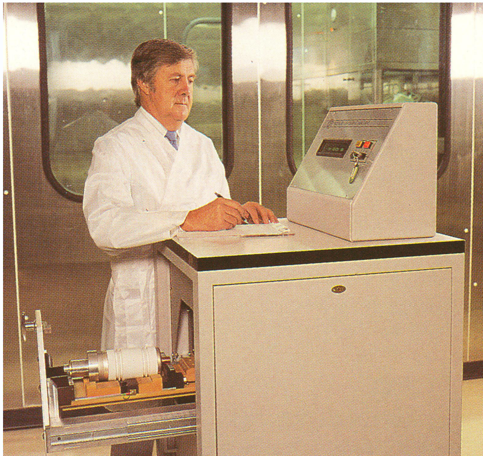
V204 interrupter being loaded into the CUPE Pressure Measuring Machine. South Africa 1990.
