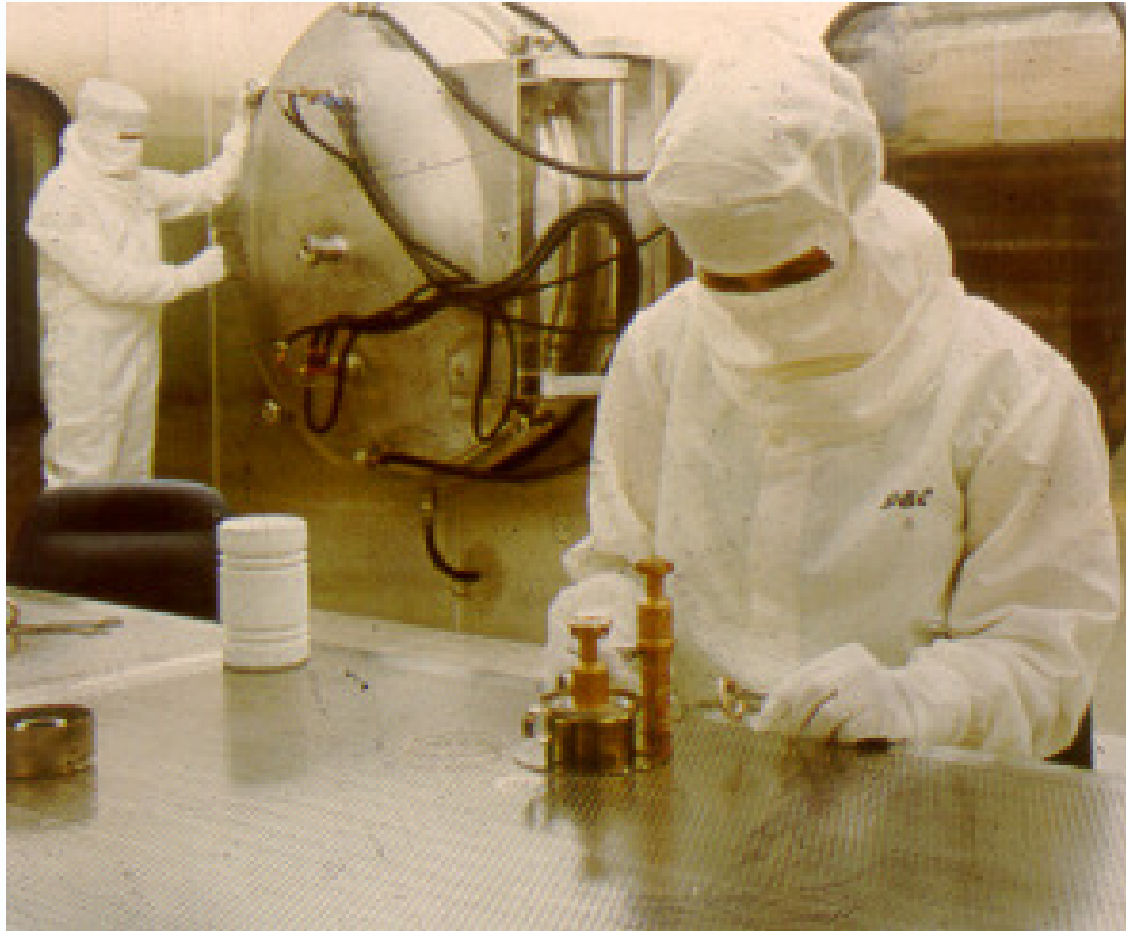
V204 interrupters being loaded into the furnace for seal off. South Africa 1990.
