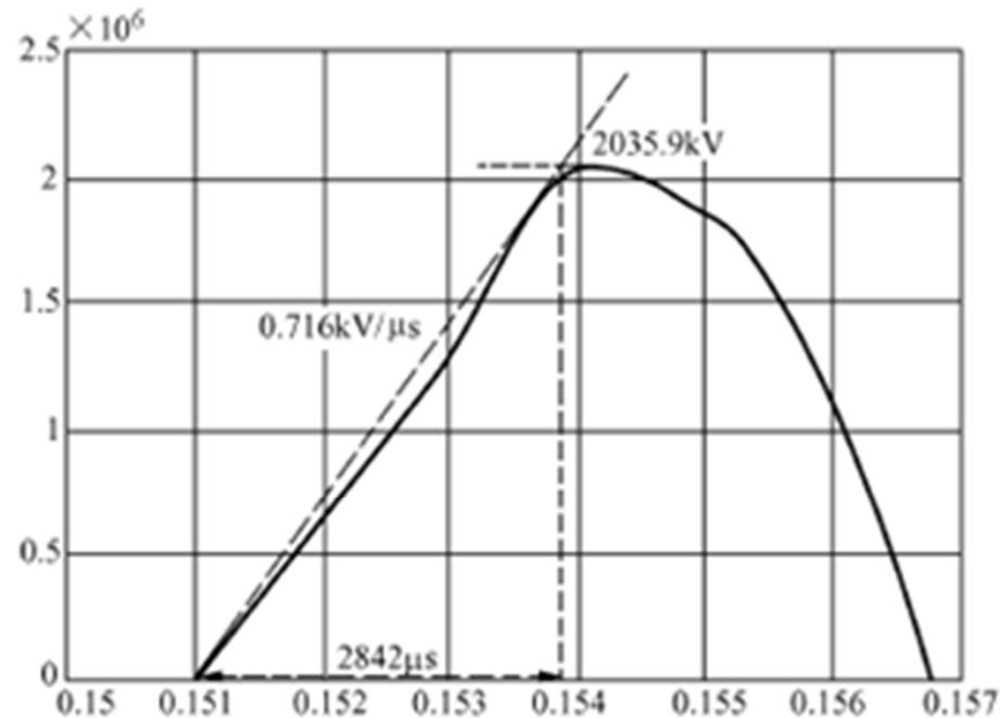
Fig. 5 TRV waveform of Nanyang CB during out-of-phase while the oscillation center is in Jing-Nan line
