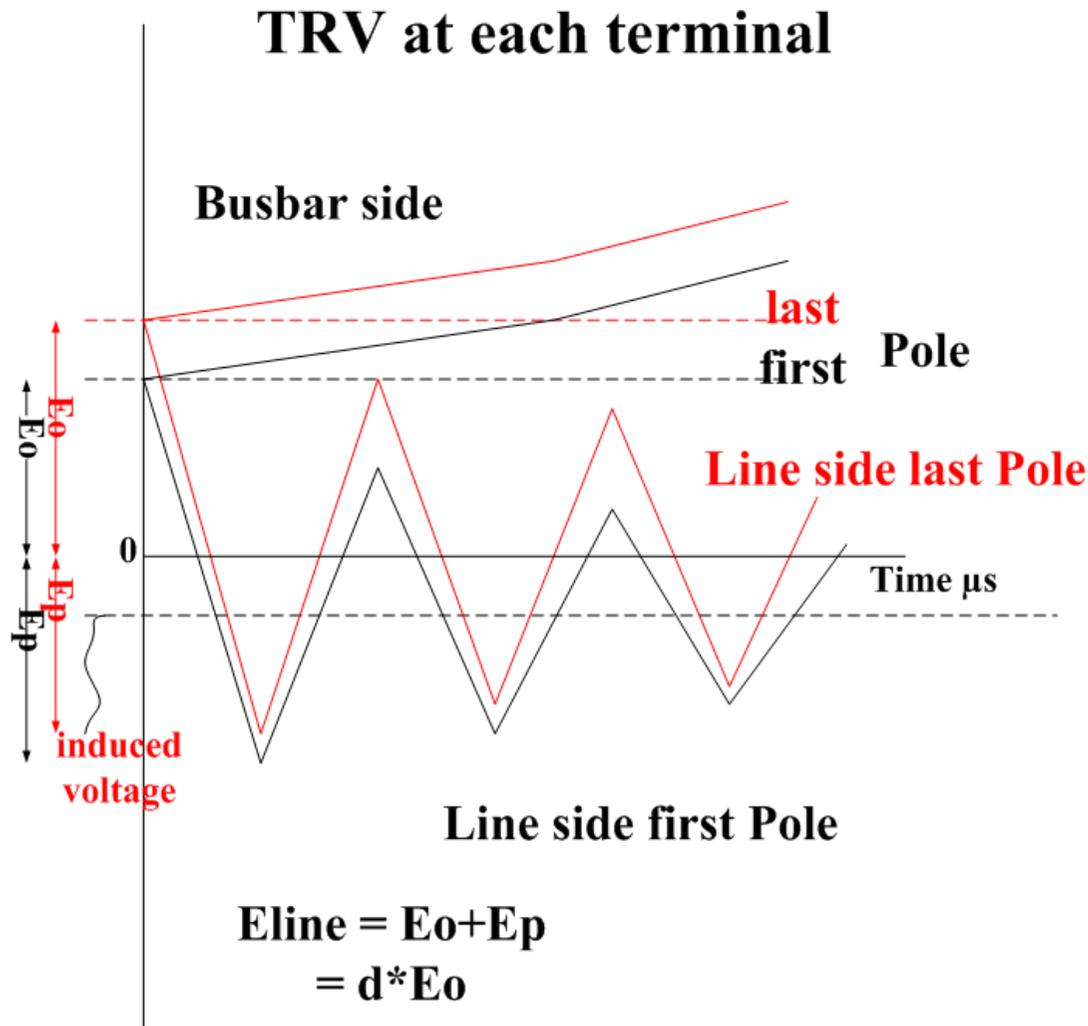
3-phase fault, first versus last pole:
