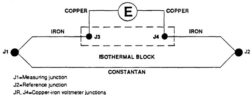
If the reference junction temperature is at 0 deg. C (in an ice bath), then, since the voltages in the tables are referenced to 0 deg. C,  $E_2 = 0$ , and  $E = E_1$ . Now, we can eliminate the summing step, and just read the temperature directly from the tables.
