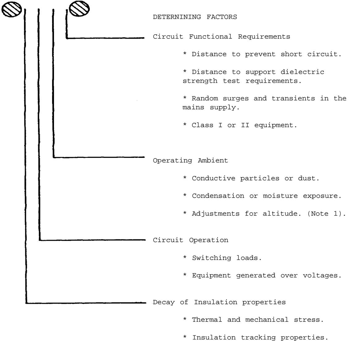
Note 1. Many standards limit spacings specified in the tables to equipment usage up to 2000 meters (6,560 feet).
