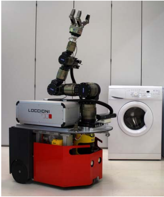
Figure 1: Mobile Inspection robot equipped with sensors and a manipulator to interact with a washing machine
