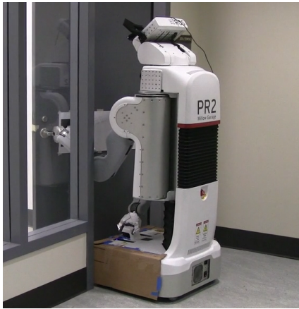
Fig. 1. The PR2 pushing open a spring-loaded door. Once the base is in contact with the door, the arm can let go of the door and use the base to keep pushing the door open as it moves through.
