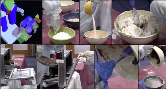
Fig. 1. A pictorial timeline of the baking process, clockwise from top left: object recognition, grabbing the ingredients, pouring ingredient into mixing bowl, mixing the ingredients, pouring the batter into the pie pan, scraping the mixing bowl, opening the oven, placing pan into oven, closing oven.
