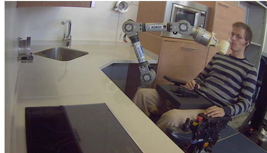
Figure 1. ASIBOT robot [1] working with a user in a real kitchen environment.
