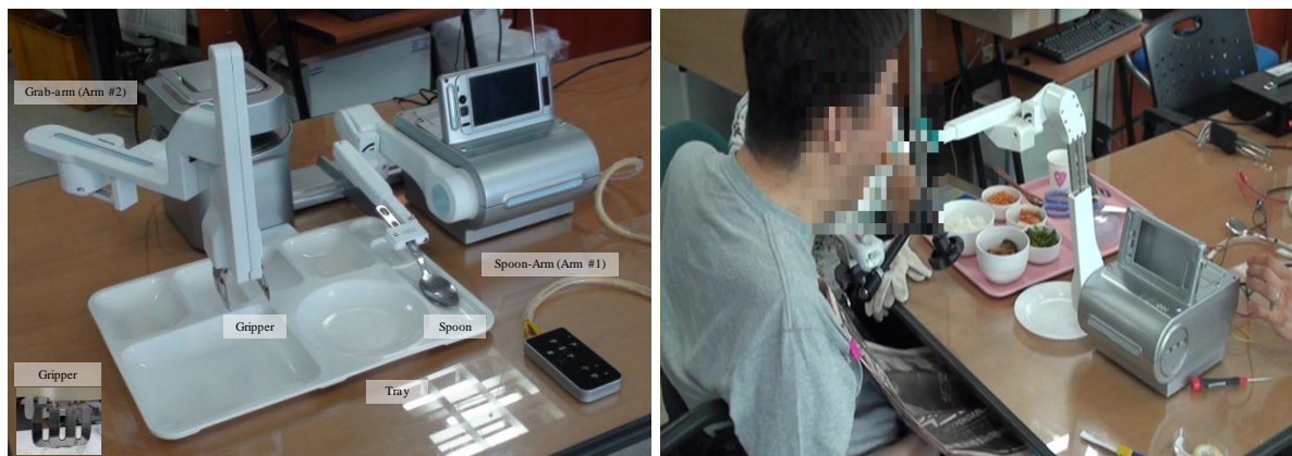
Figure 1. New assistive robot for self-feeding (left-hand side). Spoon-arm (Arm #1) uses a spoon to transfer the food from a container to a user’s mouth. Grab-arm (Arm #2) picks up the food from a container and then loads it onto the spoon of Arm #1. The self-feeding robot in a single arm configuration (right-hand side).
