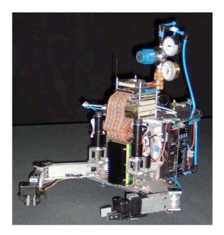
Computational autonomy is achieved with a PC104 mounted on the robot and power autonomy is achieved with a set of on-board batteries. Three optical sensors mounted at the robot base, and sourced from easily available, low cost commercial mice, provide position feedback. An external top camera also provides absolute position feedback. The position feedback system is validated with a PhaseSpace motion capture system. Using this robot, a number of experiments are possible.
