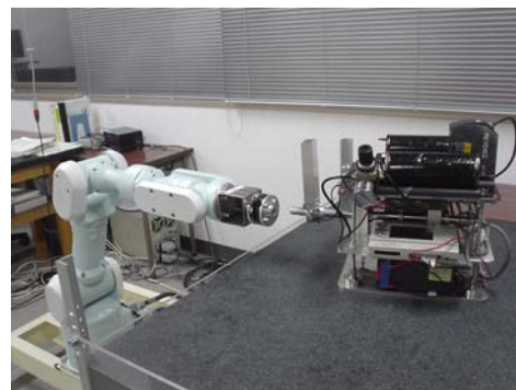
Fig.2: Target capture experiment using a free-floating test bed
