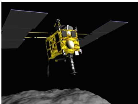
Fig.1: Touch-and-Go sampling by Hayabusa
