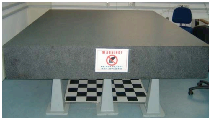
Figure 2. (a) Evolution of the robot from concept to current configuration and (b) the flat granite table.
