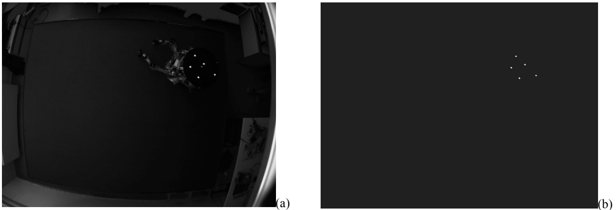
Figure 5. Frame captured by the camera: (a) before and (b) after half-toning to reveal only LEDs.
