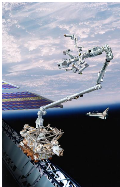
Figure: Dextre at the tip of Canadarm2 (Gonthier, 2007).
