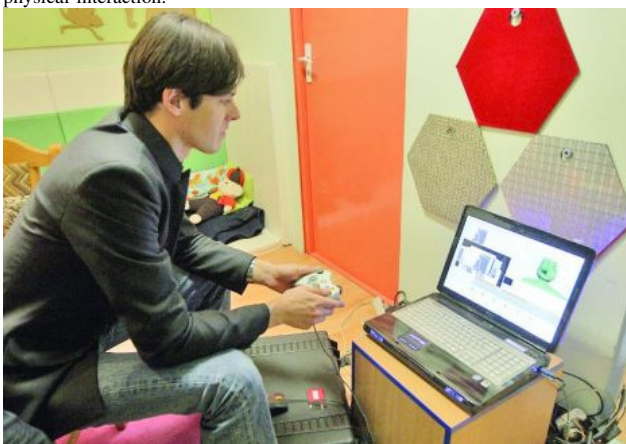
Fig. 5. The robot is used in a Wizard of Oz method, with the operator sitting in another room and using a gamepad to control the robot.
