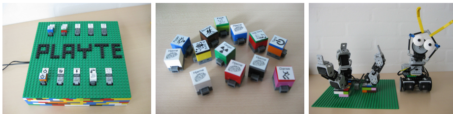
Fig. 4. (Left) The Playte: an tangible interface for behaviors-based robot control. (Center) Different predefined and trainable behavior-bricks. (Right) Example Bioloid robots that can be controlled from the Playte.
