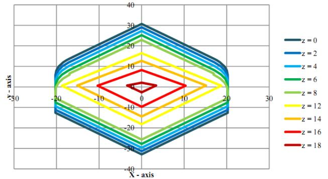
Fig. 7: Simulated results of combined lateral misalignment showing compliance within a dome-like volume. Units in mm.
