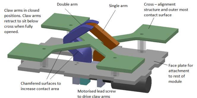
Fig. 1: The X-CLAW connector design.
