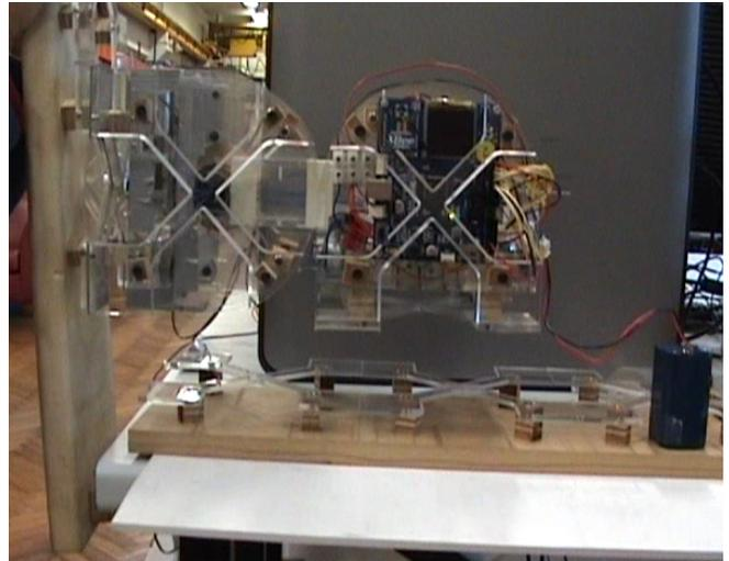
Fig. 8: Retention testing of the connector in one of the more challenging configurations to maintain connection for due to the large moment arm.
