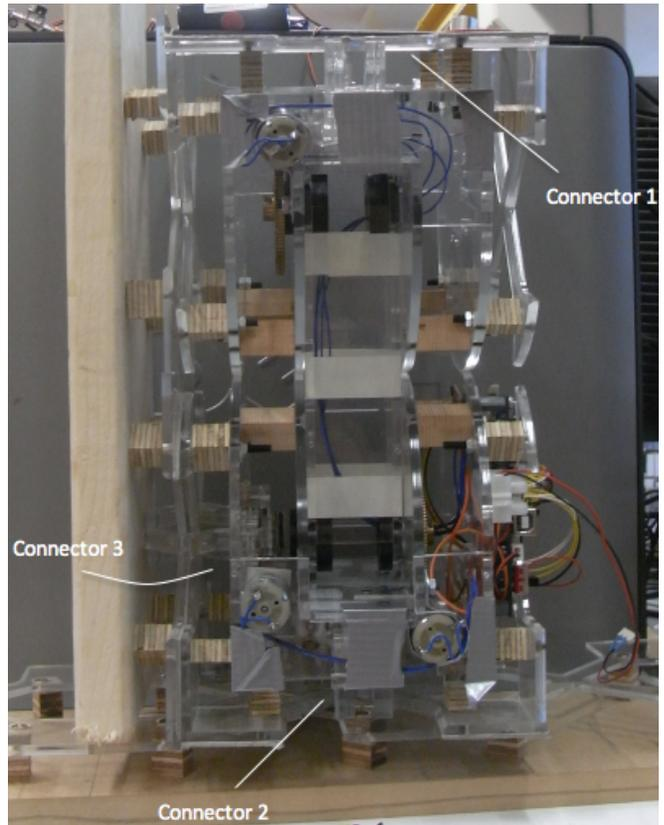
Fig. 6: Test module with three active connectors installed. This is sufficient to perform tests demonstrating compliance and strength.
