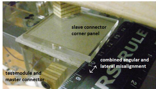
Fig. 10: Observed translational freedom between docked connectors. Maximum offset of  $6 \text{ mm}$  was measured at corners.
