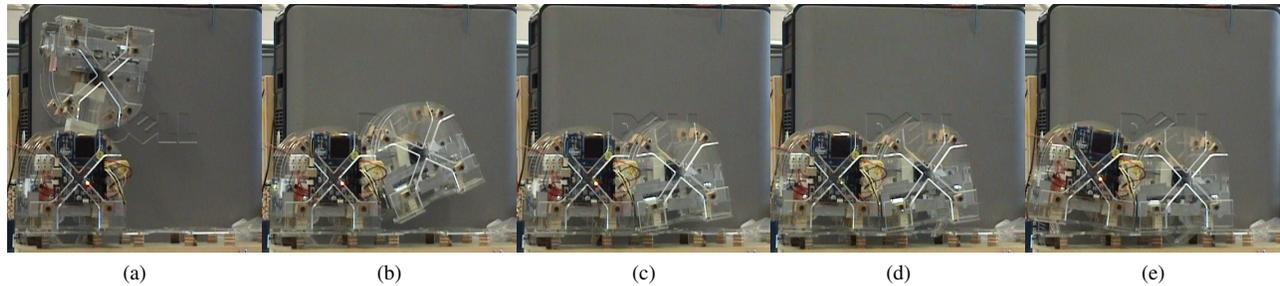
Fig. 9: Test module shifting connection between connectors on simulated lattice. Angular misalignment is introduced by artificially limiting joint range.
