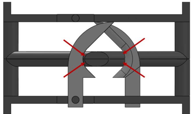
Fig. 3: Claw prismatic profile in contact with complying surface on cross: the horizontally applied forces are translated into a vertical ones, compressing the contacting crosses together.
