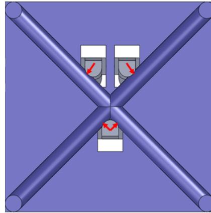
Fig. 2: Claw-cross arrangement: vertically opposite forces applied by arms to cross forcing the cross to center.
