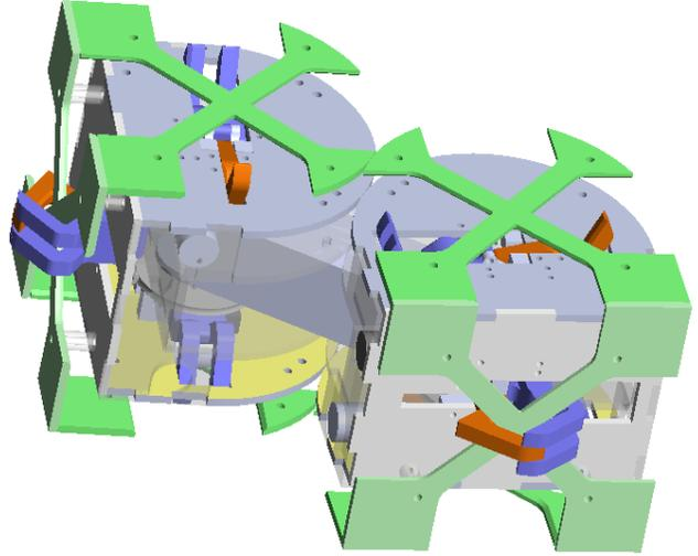
Fig. 5: CAD model of test module with six connectors installed.
