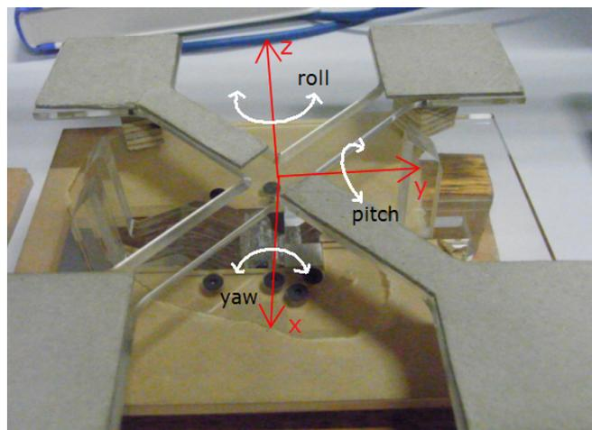
Fig. 4: Connector prototype and the six degrees of freedom in connection: three lateral, three angular.
