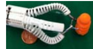
prototype for endoscopic interventions with the spine-inspired kinematic structure actuated with push rods
