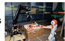
Figure 6. Robot to robot interaction scenario where NAO points at red wooden car and Kinova's JACO arm grasps and relocates the object.
